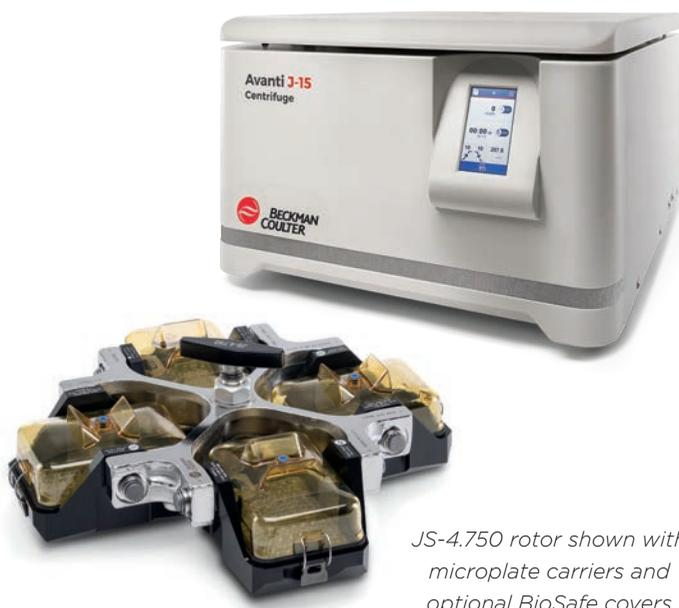
*JS-4.750 rotor shown with microplate carriers and optional BioSafe covers*
